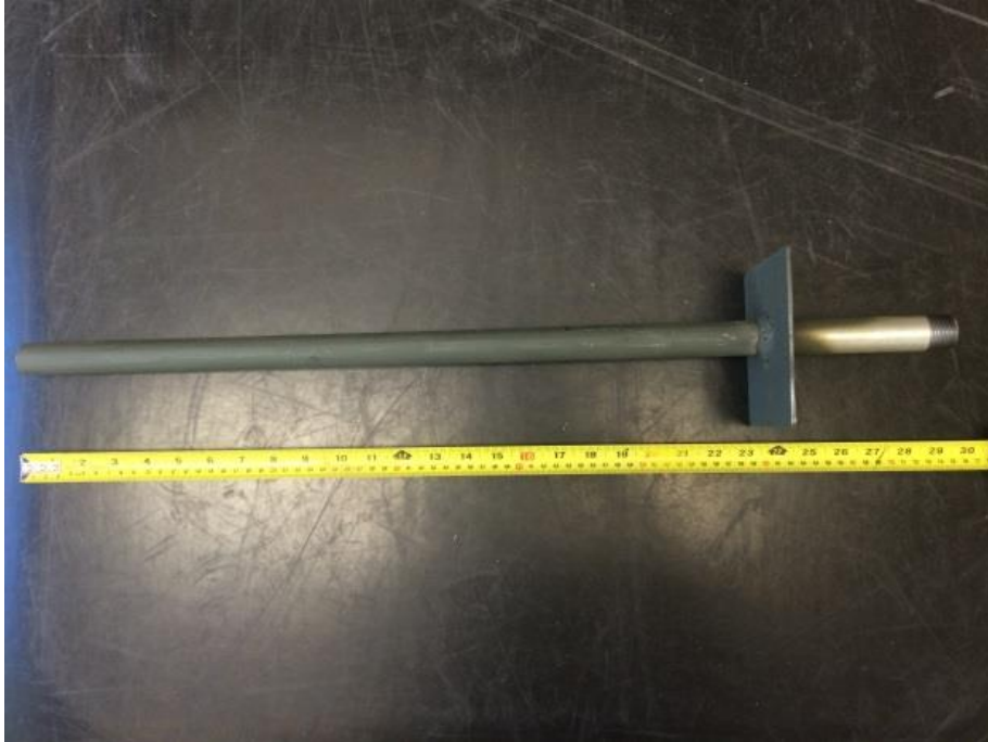
Figure A 18. Photograph of mounting arm assembly with welded steel plate.
