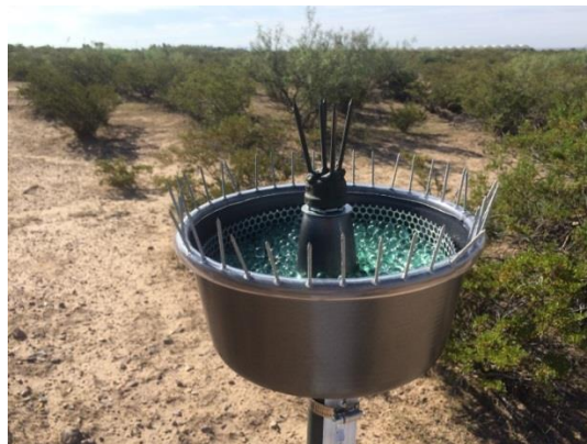
Figure A22. Dust deposition trap mounted in the field.
