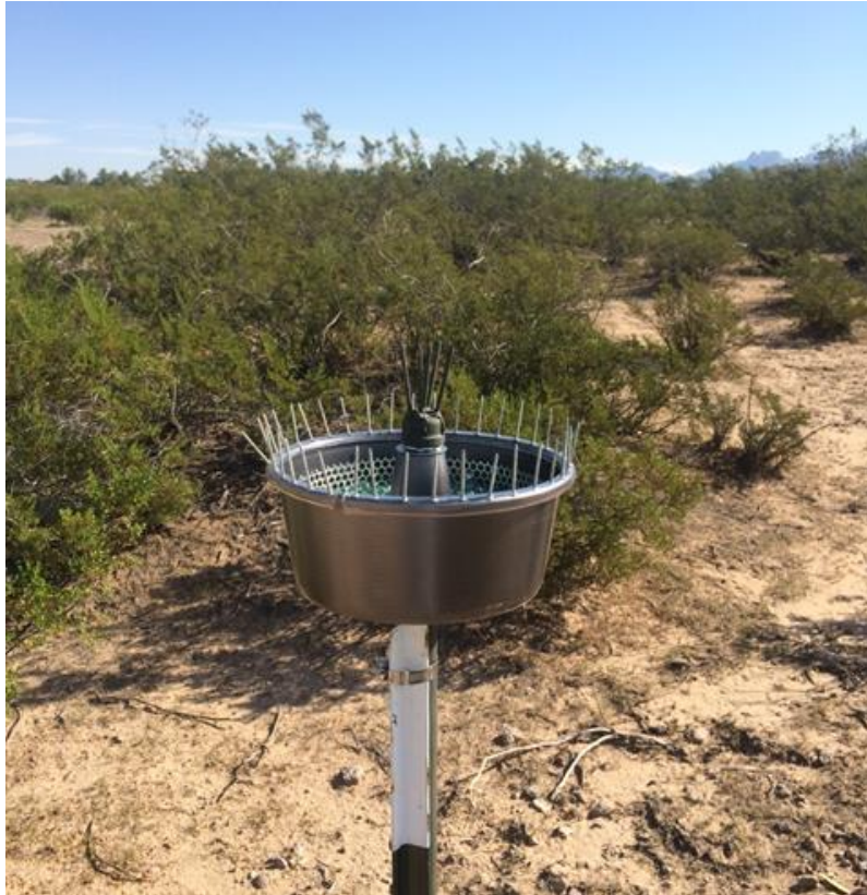
Figure A23. Dust deposition trap mounted in the field.
