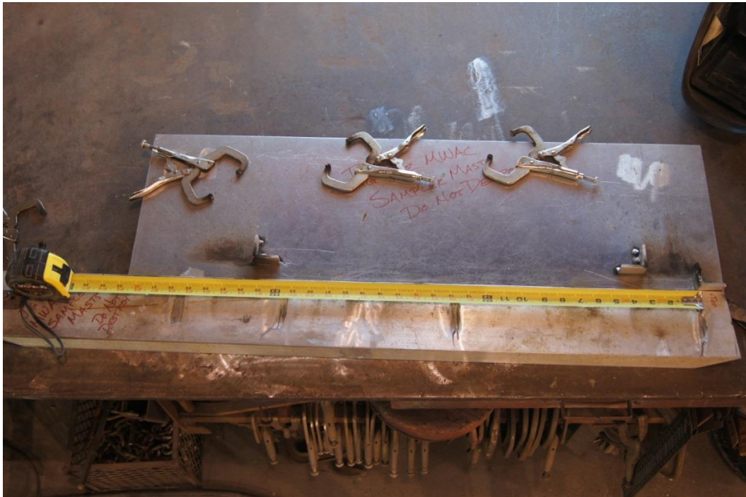
Figure A5. View of jig for welding retainers for hose clamps and fin to mast. Note: Figure A6 shows mast with fittings positioned in jig.
