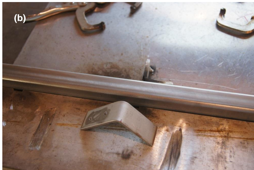
Figure A7. Upper (a) and lower (b) fin supports with holes drilled to attach the top and bottom aluminum right angles and fin.
