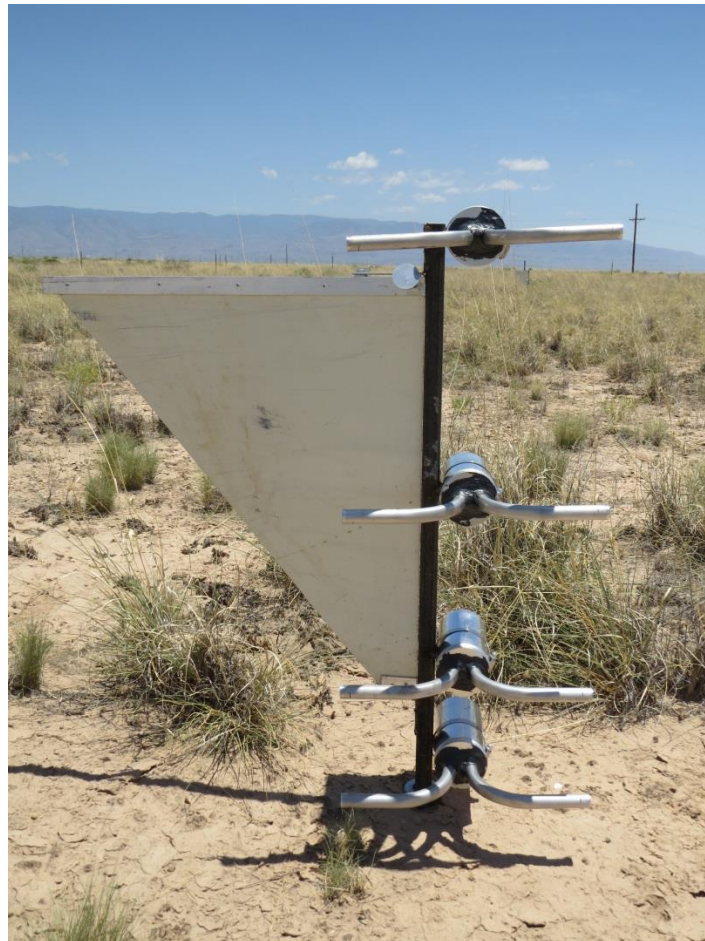
Figure A17. MWAC mast with four samplers installed in the field.
