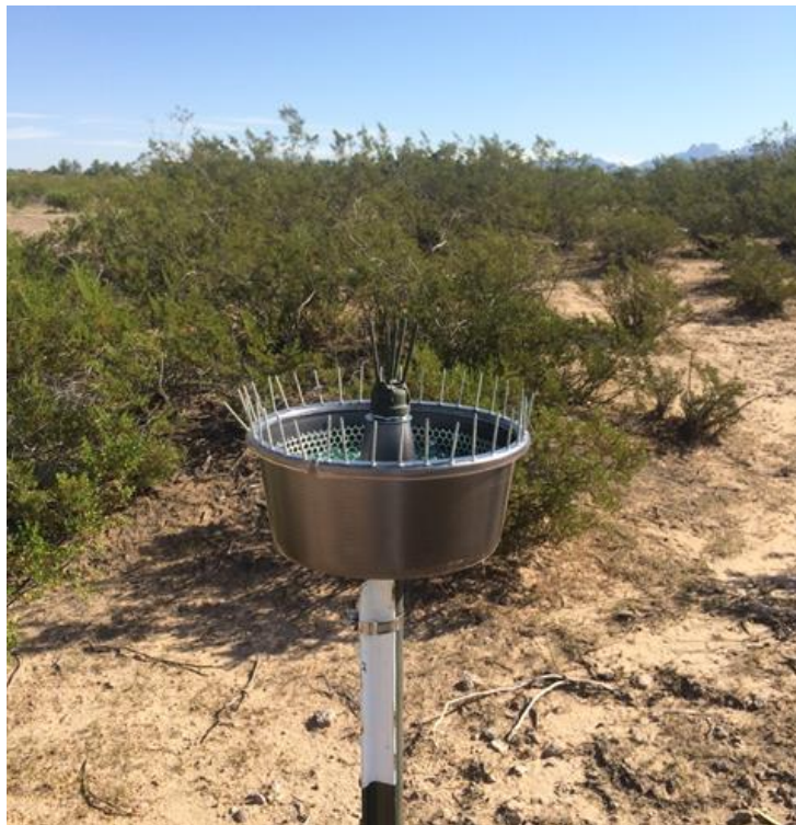
Figure 13: Photograph of a dust deposition trap (e.g., Reheis and Kihl, 1995) deployed in the field.
