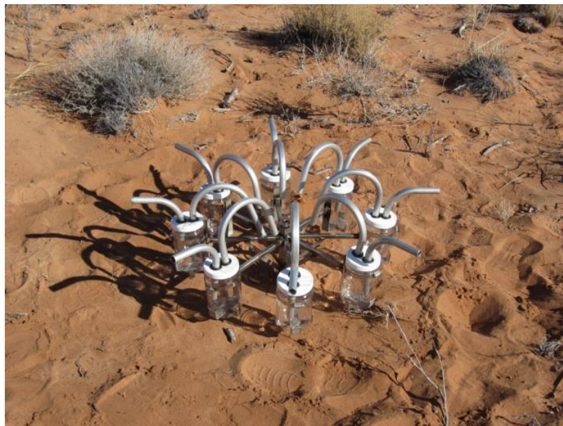
Figure 12: MWAC samplers deployed on a directional bracket to sample sediment flux from the four cardinal and four intercardinal directions (N, NE, E, SE, S, SW, W and NW).
