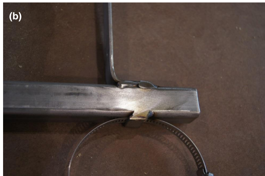
Figure A10. Welded MWAC mast (a) and close-up of the top welded hose clamp and fin support (b).
