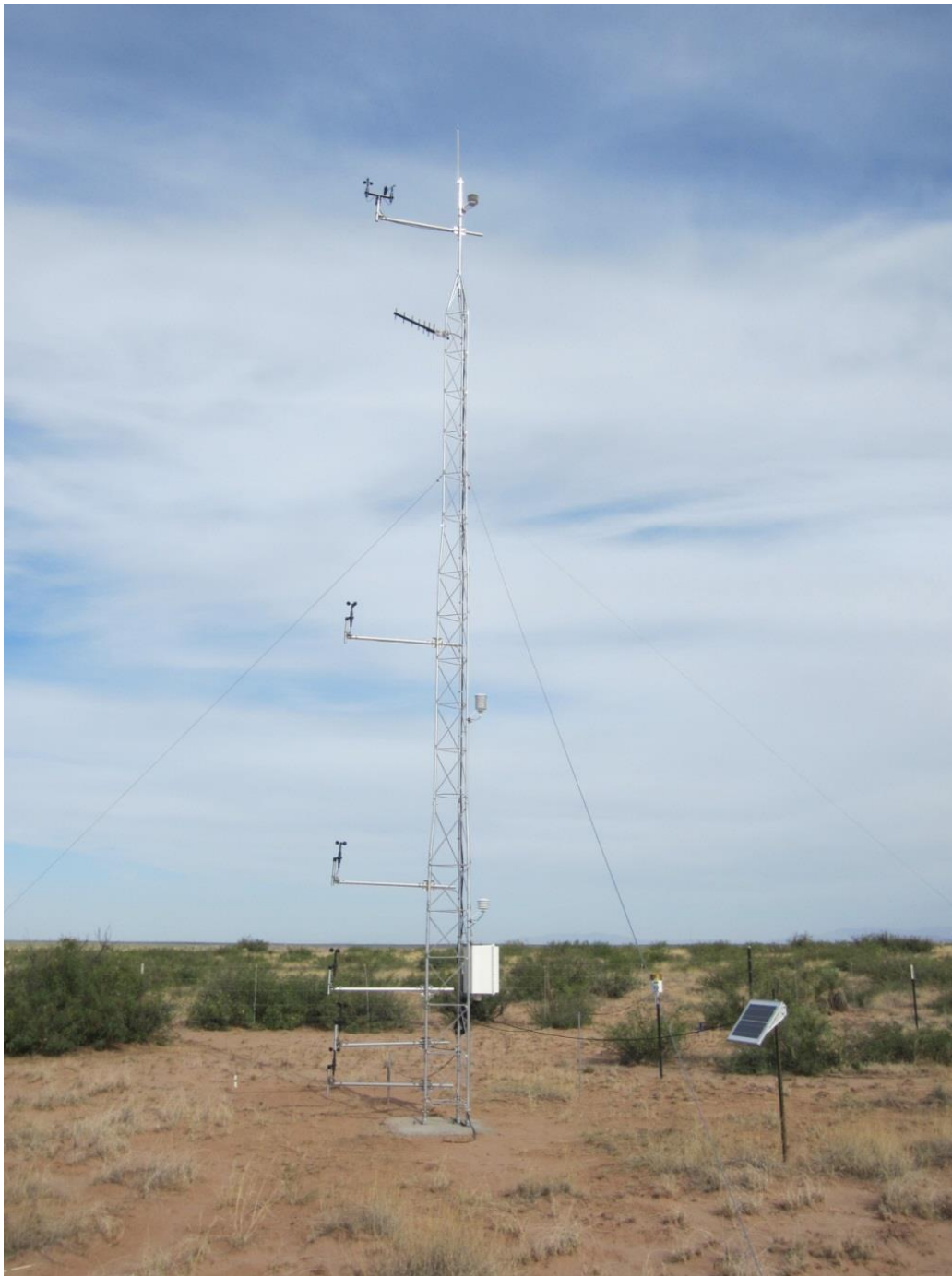
Figure 4: Photograph of instrument mast on which are mounted the six anemometers (plus one wind vane at top), three air temperature sensors and relative humidity sensor (on right of tower), data logger enclosure, solar panel (may also be mounted on tower), rain gauge (at rear), Sensit (in ground, left of lowest anemometer), and communications antenna (facing direction of nearest cell phone tower).
