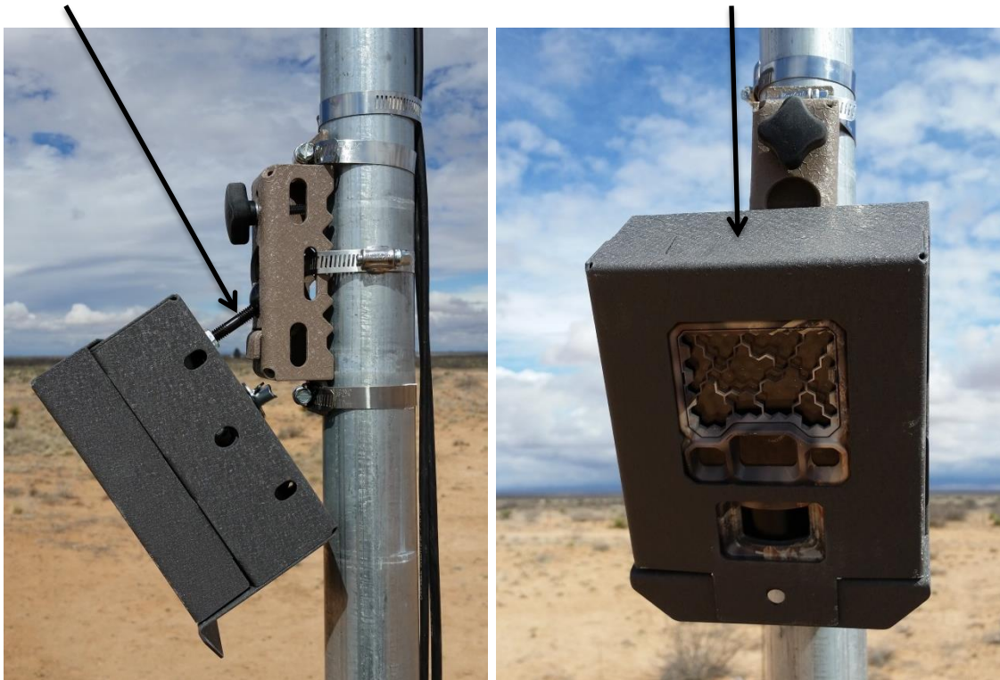
Figure A3. Photograph showing time-lapse camera mounted to mast with ball-arm for adjusting camera enclosure, in which the camera is contained.
